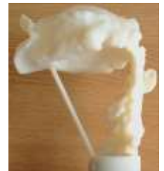
A 3-D print of a vocal tract for an adult male "ah" vowel as used in the Vocal Tract Organ.
